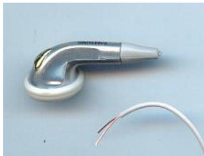
2. Then use the appropriate tool to peel off the superficial rubber protector of the wire, after which two strands of different colors thin wires will be revealed, each strand is composed of dozens of or to several hundred very thin enamel-insulated wires (as shown in the above chart). If have no special tool
